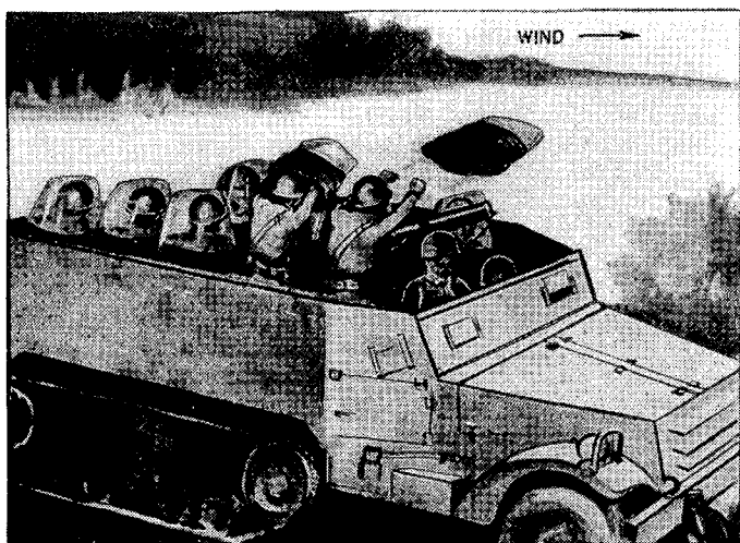
FIGURE 20.—Men on up wind side remove covers successively, commencing with the man in front, and throw them over the down wind side.
