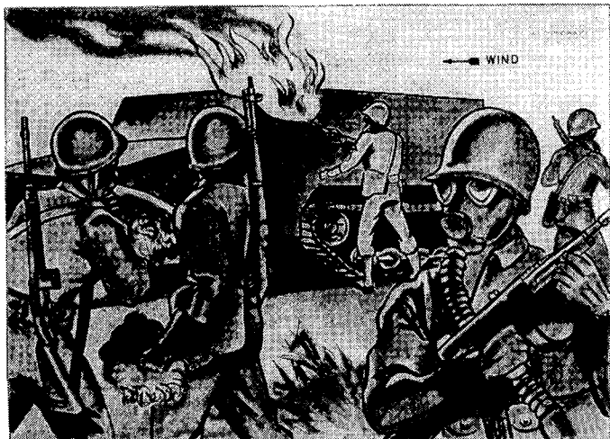
FIGURE 27.—During burning-off process crew stands up wind. Burn off a small panel at a time.
